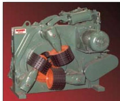
18" model with mechanical feedroll drive.
