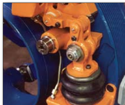
Detail of air-bag tensioning system.
