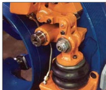
Detail of air-bag tensioning system.
