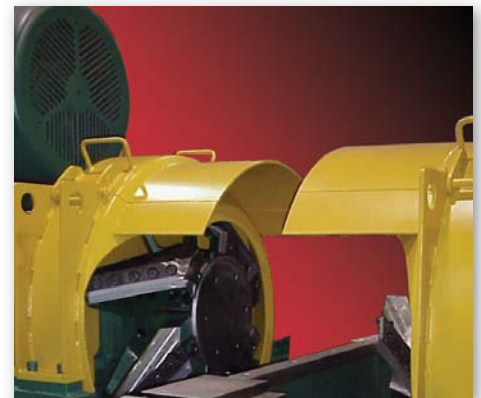
The system uses conical chip heads and VFD's to produce uniform chips at high speeds
