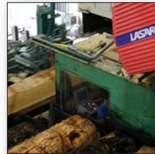
▲ The LASAR™ sensor scanning on the fly in a headrig carriage application
