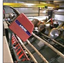
▲ The LASAR™ sensor in a bucking application
